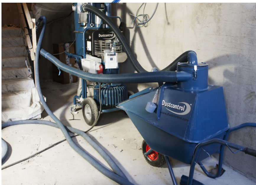
DC 5900, 9.2 kW P central unit with DC F Wheelbarrow pre-separator.
